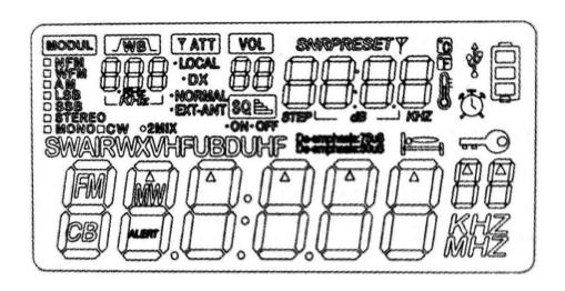
MODUL: Modulation mode switching display
